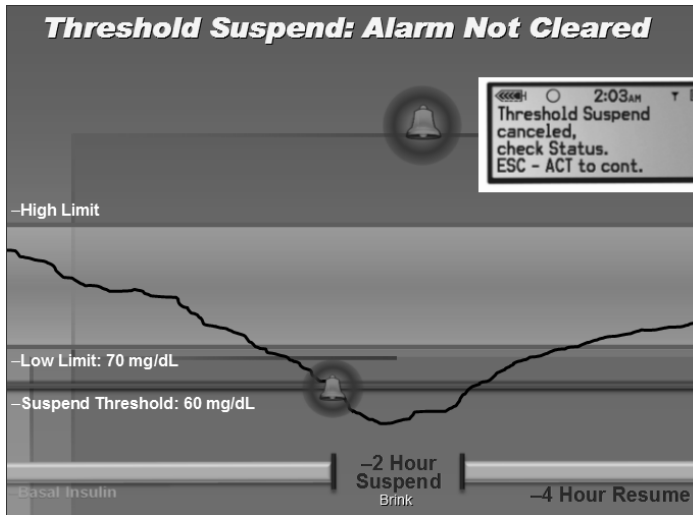
Figure 5.17: Threshold Suspend diagram documenting actual CGMS glycemic results with 2 hour LGS after no response to decelerating glycemia (black line), no response from 70 down to 60 mg/dl (blue to purple lines) suspend threshold (shown with cessation of gold basal insulin bar) and then the automatic 2 hour suspend and resumption of insulin delivery thereafter.
